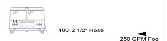
400' of 2  $\frac{1}{2}$ " hose<br/>GPM = 250FLR =2 $Q^2$ Q = GPM / 100FLR =2 x 2.5^2Q = 250 / 100FLR = 2 x 6.25Q = 2.5FLR = 12.5 -round to a whole numberFLR = 13TFL = FLR x LL = Lay / 100TFL = 13 x 4L = 400 / 100
