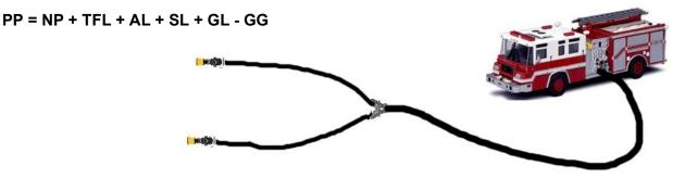
Before the FLR formula can be solved the GPM must be converted to the equivalent flow for all the hose in the lay other than  $2\frac{1}{2}$ ". The flow through the  $2\frac{1}{2}$ " hose is the figured as the actual total GPM.
