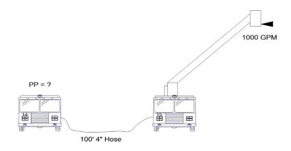
PP = Initial Aerial Pressure +/- Adjustments GPM = 1000
